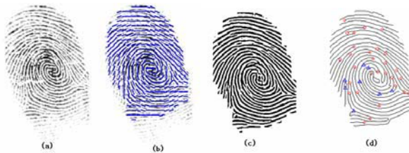
Fig. 1 Fingerprint preprocessing.(a)An original fingerprint in DB1_Aof FVC2004,(b)its block orientation field,(c)enhanced image,(d) thinned image of fingerprint image
